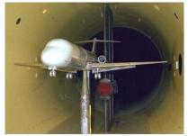
model 1:4 must be tested at four times the real speed. Hence the smaller the model, the higher the speed in the test section, this is called the scale-effect.
