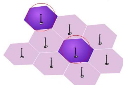
nearest base station. If you travel through the different cells the mobile phone automatically connects to the nearest base station again. The reach of a mobile phone is up to 8 kilometres.
